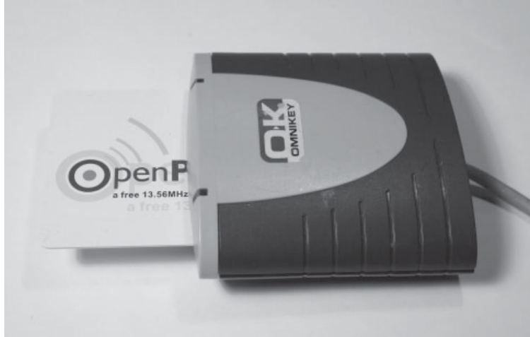
Figure 10-8 OpenPICC smartcard reader
