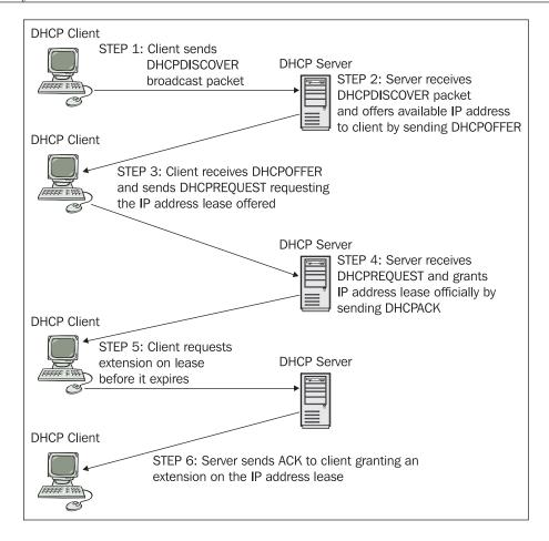
The DHCP server gives the IP address to a requesting device on a lease basis, meaning that the IP address is "leased" for a limited amount of time. During this time, the DHCP server will not lease that IP address to any other clients. Before the lease time expires, the DHCP client must request an extension of the lease time from the DHCP server. The DHCP lease time is configurable from 120 seconds to whatever the administrator chooses.
