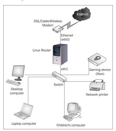
The provider usually assigns us a public IP address that can be either statically assigned or dynamically assigned using DHCP or PPPoE. Linux has support for PPPoE; this can be downloaded from http://www.roaringpenguin.com/pppoe/.
