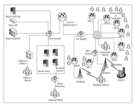
Core-4 is a Linux router that handles a lot of network traffic. It has six network interfaces, three of them connected to the other core routers, two connected to a core switch in Datacenter-4, and one to the fiber optics switch also located in Datacenter-4.
