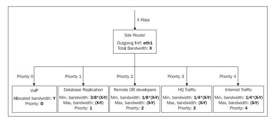
To differentiate these services we will mark packets in the mangle table in the POSTROUTING chain for every service, using the MARK target of iptables (module ipt MARK).
