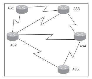
A provider having the Autonomous System number 1 (AS 1) has two interconnections: one with AS 2 and another with AS 3. Depending on the agreement between the providers, AS 1 can route to either of them only their own networks (Local Exchange or Local Peerings), or it can announce all the routes received from other peers (Full Exchange or Full BGP).
