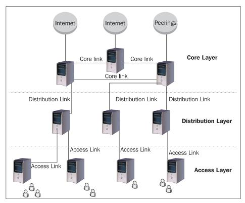
The core layer usually contains routers that have internet or local peering connections. There are high-speed links between them, and routes are distributed between them for better load balancing of internet and peering connections.
