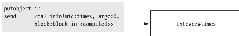
Figure 6-8: The YARV instructions on the left should call the implementation of Integer#times on the right.
