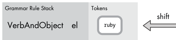
Figure 1-23: The parser shifts another token onto the stack.
