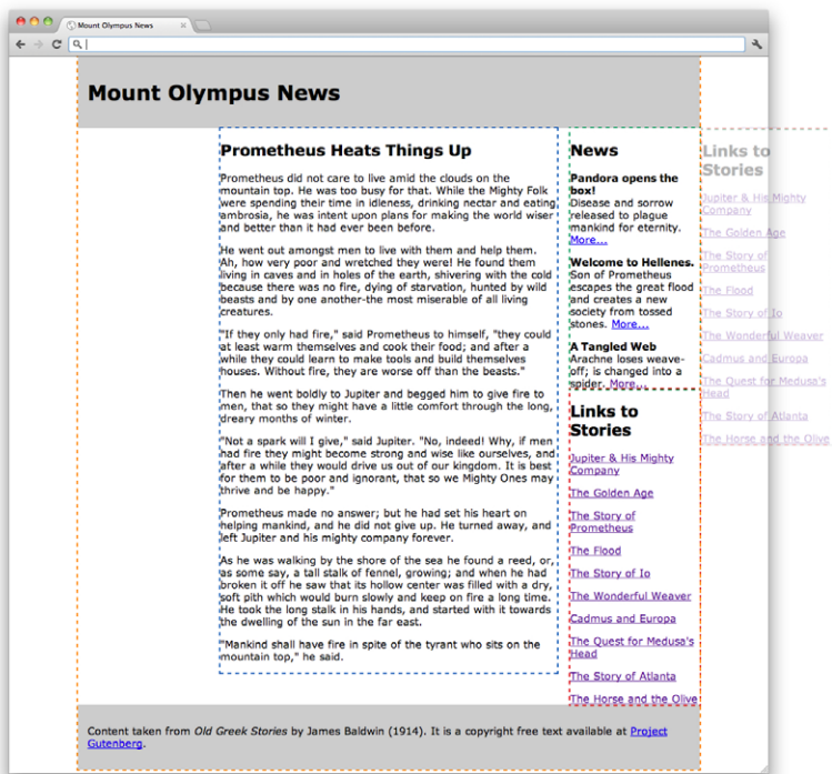
Figure 16-14. The layout after margins are applied to the middle ( #main ) column element. The shaded box on the right shows where #links would like to be if it weren't forced under #news .
