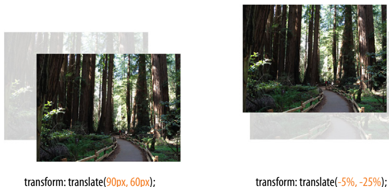
Figure 17-9. Moving an element around with the translate function.
