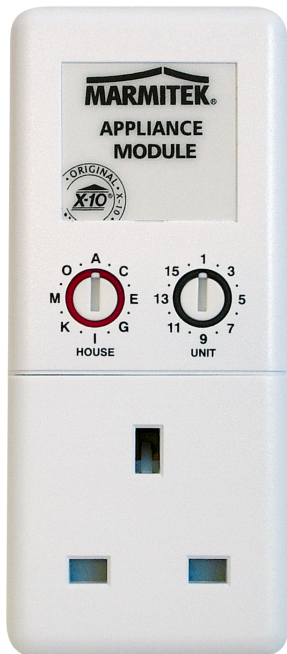
Figure 1-7. The AM12U, 52 ×122 ×33mm
