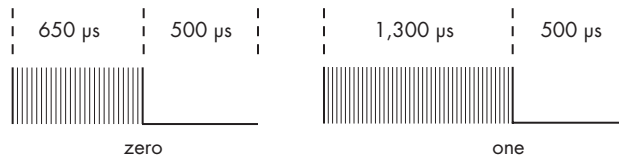
Figure 12-3: Modulated pulses in the Sony TV protocol
