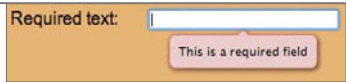
FIGURE 2.7 Error message for the text input type when it is not filled in before submission.
