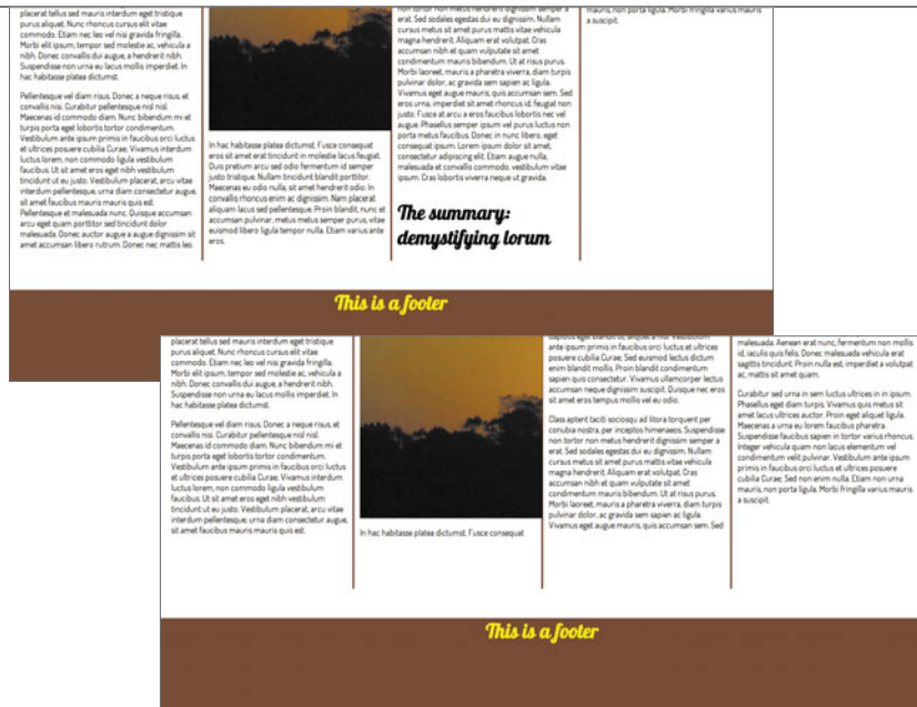
FIGURE 7.4 Demonstrating the difference between auto column fill (left) and column-balanced column fill (right).
