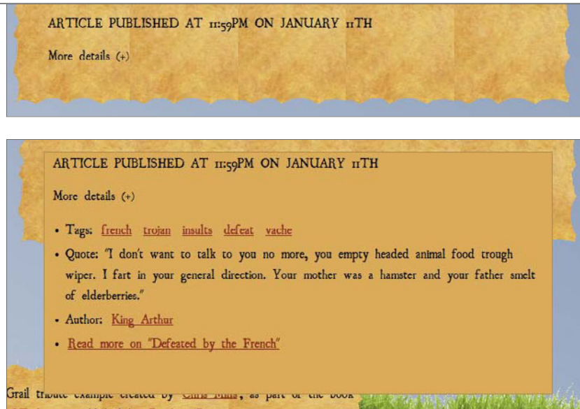
FIGURE 5.21 A CSS Transition is used to smoothly animate between “closed” and “open” footer states for the Monty Python blog example.
