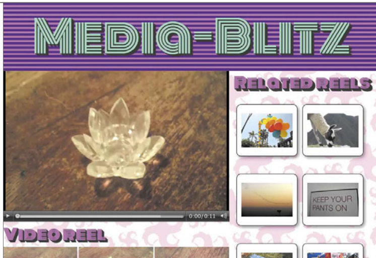
FIGURE 8.8 The result of the first media query kicking in. The navigation menu moves from the side of the site down to the bottom, and the rest of the content expands to span the entire width of the browser.
