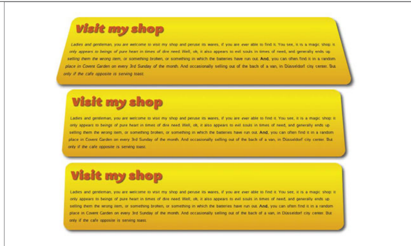
FIGURE 5.10 The effect of different perspective transform values on a simple rotateX transform.
