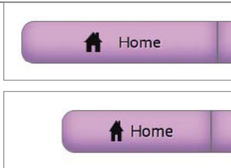
FIGURE 6.14 Using background-size to scale the icons proportionately to the size of the menu buttons.
