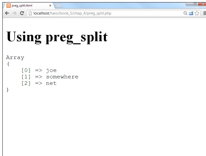
Figure 4-9: The e-mail address split into an array.
