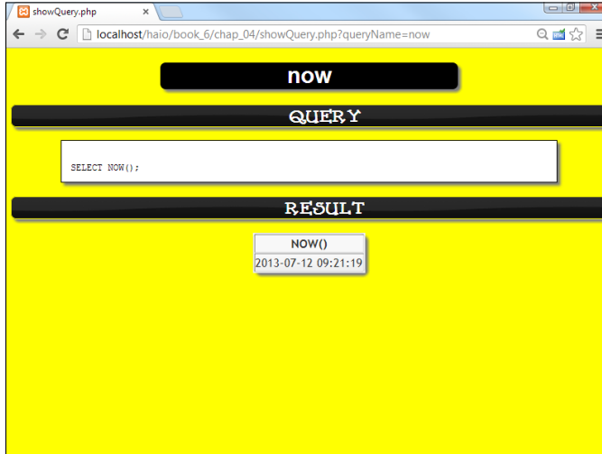
Figure 4-2: The NOW() function returns the current date and time.
