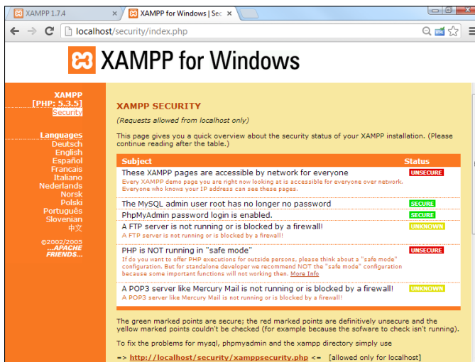
Figure 1-4: The XAMPP Security panel shows a few weaknesses.
