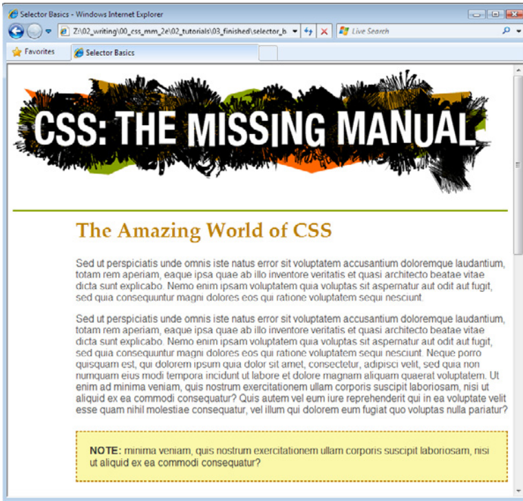
FIGURE 3-12 You can make detailed formatting changes with class selectors. A class style gives selected paragraphs different formatting from all other paragraphs on the page. The distinctive note box pictured here uses a class style to stand out from the crowd.
