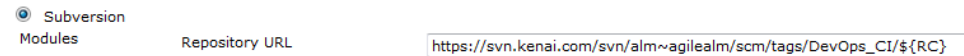
Figure 8-6. Configuring Jenkins to check out the baseline that is defined by the user on runtime.
