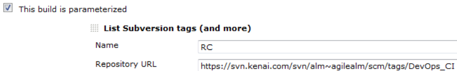
Figure 8-5. Configuring a parameterized Jenkins build job that will offer a combo box of existing Subversion tags under the defined path. The concrete one (in our case, expressed by the variable RC) is available in the Jenkins build job afterward for further processing.
