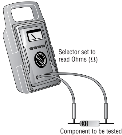
FIGURE 2.11 Connecting a multi-meter to measure resistance
