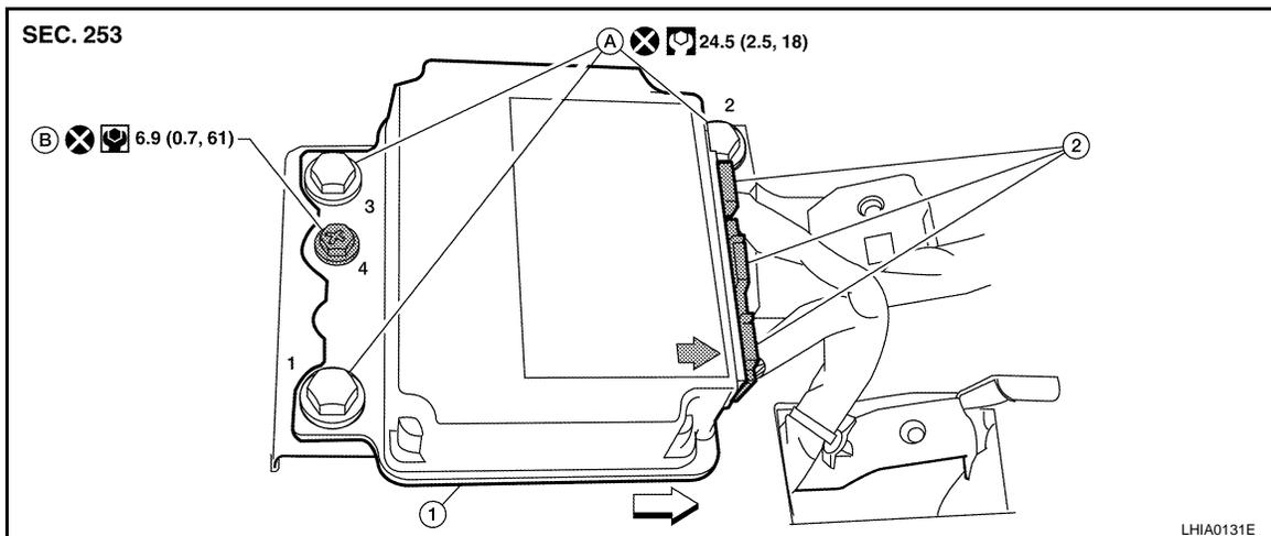
1. Diagnosis sensor unit                      2. Diagnosis sensor unit connector                      A. Diagnostic sensor unit bolt
