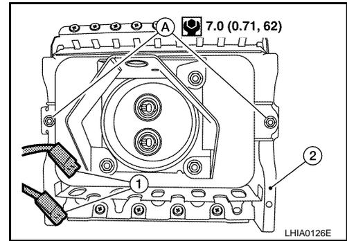
5. Install the front passenger air bag module lower bracket bolt (A) to the steering member (1) through glove box opening.
