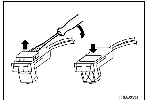
5. Disconnect horn connector (1) and release harness from clips (2).
