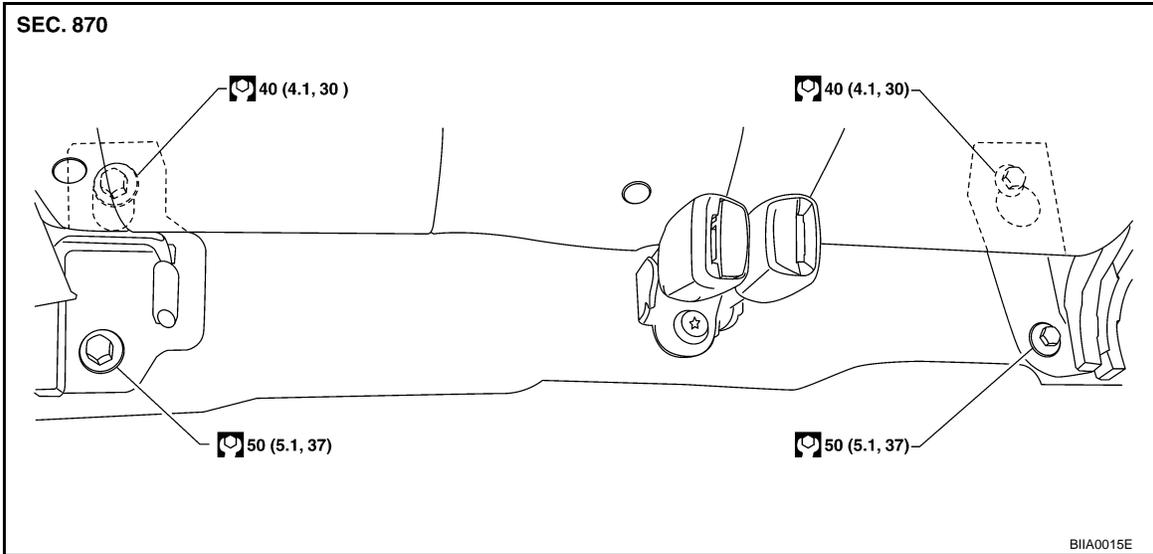
2. Remove the lower seatback mounting bolts from the right rear seat back brackets.
