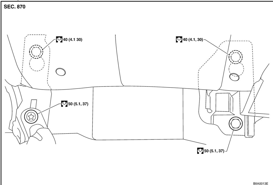
2. Remove the lower seatback mounting bolts from the right rear seat back brackets.
