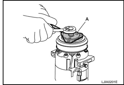
4. Remove the snap ring using external snap ring pliers.
