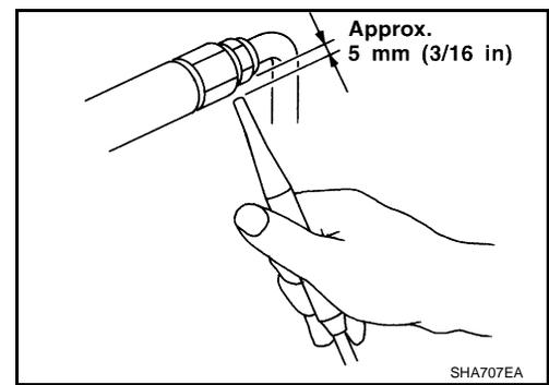
2. When testing, circle each fitting completely with the leak detector probe.
