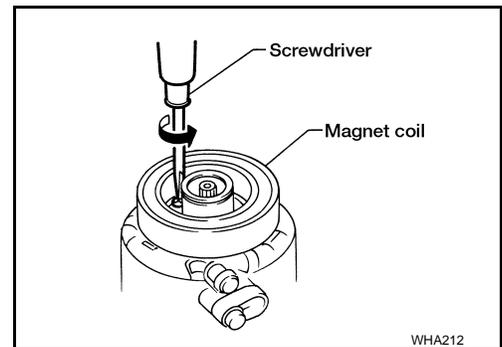
8. Remove the three magnet coil screws and remove the magnet coil.
