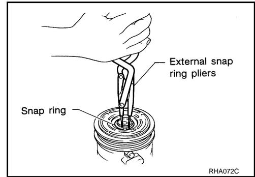
5. Remove the pulley assembly using Tool.
