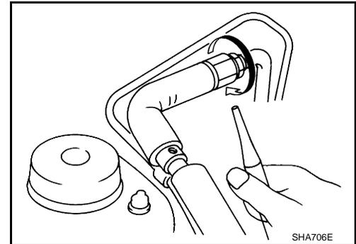
3. Move the leak detector probe along the component at approximately 25 to 50 mm (1 to 2 in)/sec.
